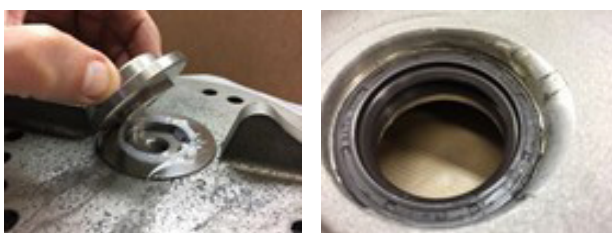
Both photos show the end shield (1/13 with the mounted seals, 2pcs.) from its lower side which will face the motor.
