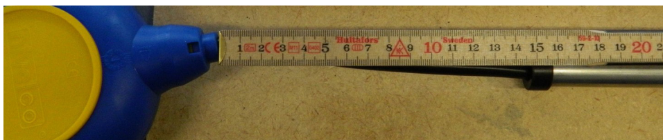
Suitable mounting length of free cable is 15cm outside the float bracket.
